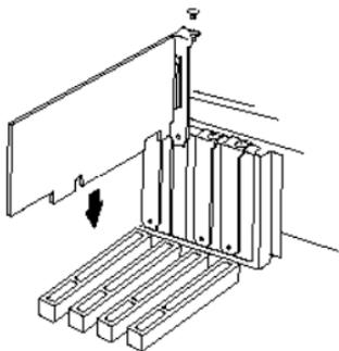
**Figure 14. Installing an Adrenaline SCSI Scanner Controller**
